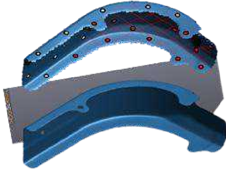
Figure 6. Scans comparison generated with 3.00 mm and 0.35 mm of resolution.
